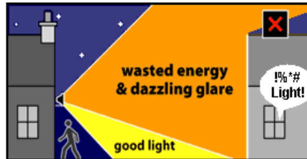
BADLY AIMED 500W HALOGEN FLOODLIGHT
