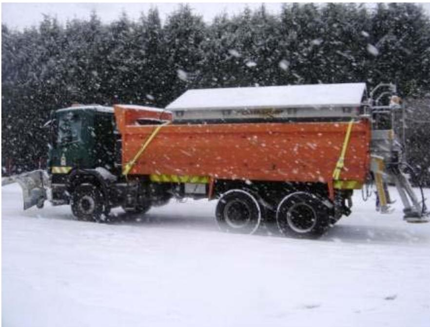
Figure 4: Demountable salt spreader
